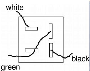
The white wire connects to one plus pin. The black wire connects to the other minus pin. The green wire connects to a plus and a munus diagonally.
