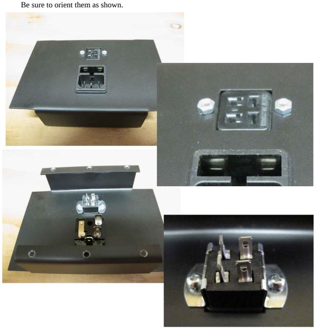
2. Mount the power supply modules to the panel with M3 8mm screws. Note that the panel is not symmetric To identify which side to mount on, measure the distance from the mount hole to the top edge. The one on the left is 2.0 inches. The one on the right is 1.9 inches.
