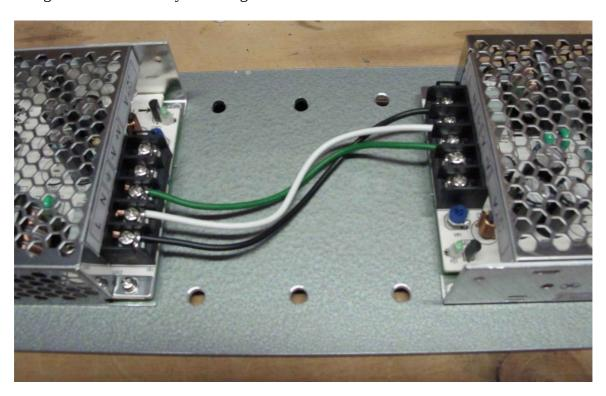
5. Attach the other wires as shown. For now, leave the other end hanging. Tighten the screws. Match the colors:
